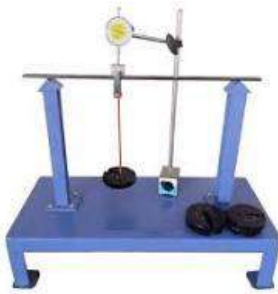
Figure 2: Simply Supported Beam Setup
